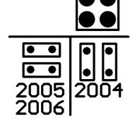
When the jumper consists of four pins in a square, correct selection is made by positioning the two jumpers in either vertical or horizontal orientation.
