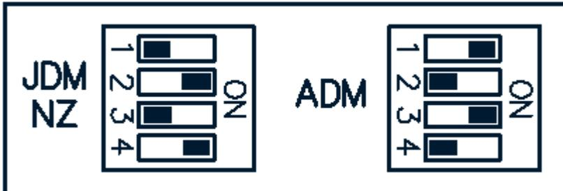
If your ECU bottom board is version 1.2 or higher, you will have a second set of jumpers. The jumpers are used to configure the board for either a 1991 - 1993 or a 1994 - 2002 SR20DET.
