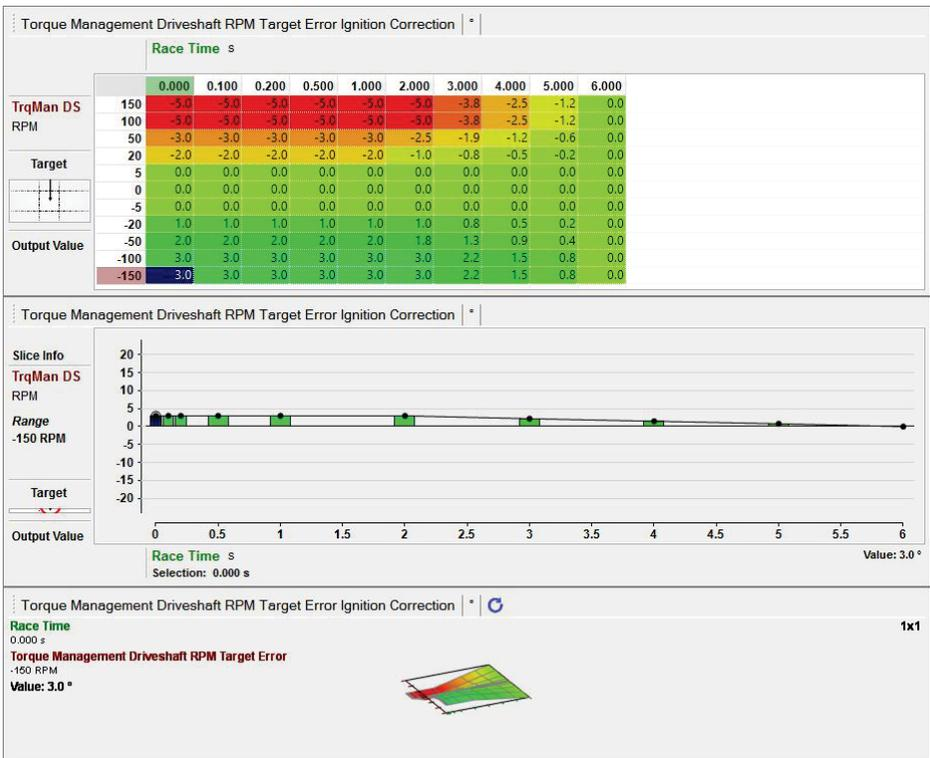
Figure 13 - Driveshaft RPM Target Error Ignition Correction table
