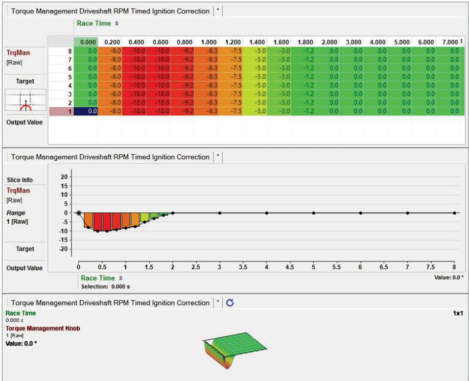
Figure 10 - Timed Ignition Correction table
